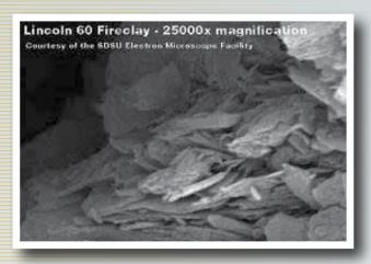
oxygen (O2) or hydroxide (OH) and a central cavity hold by a cationic or positive charge element (Si, Al, Fe, Mg) to balance forces and stabilises the structure.
